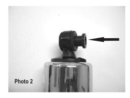
Install a shouldered sleeve as shown into each mounting eye of both shocks
