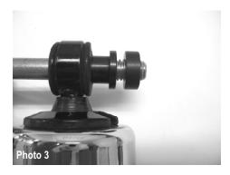
On 1991 - Later Sportsters also use one additional spacer in conjunction with the shouldered sleeve to provide sufficient space between the shocks and the Frame / Swing arm.
