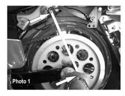
Do Not complete your Slammer Shock installation until you have checked to be sure you have adequate Tire / Fender clearance.
