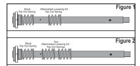
Prior to installing your Slammer Fork Lowering kit, you **MUST REMOVE** any previously installed fork lowering kit components, such as the 1 or 2 additional top out springs illustrated above. Additional top out springs are common in many such kits.
